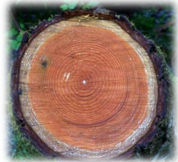
Figure 1. Cross section of Douglas-fir. Light colored outer rings are sapwood. The dark wood in center is the heartwood.
