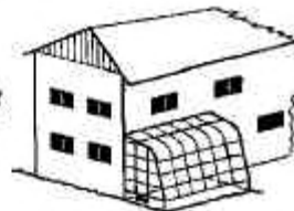
This is an example of a curved-eave lean-to built on a two-story house.
