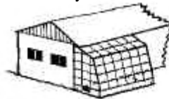
A straight-eave lean-to greenhouse can fit under the roof of a single-story house.
